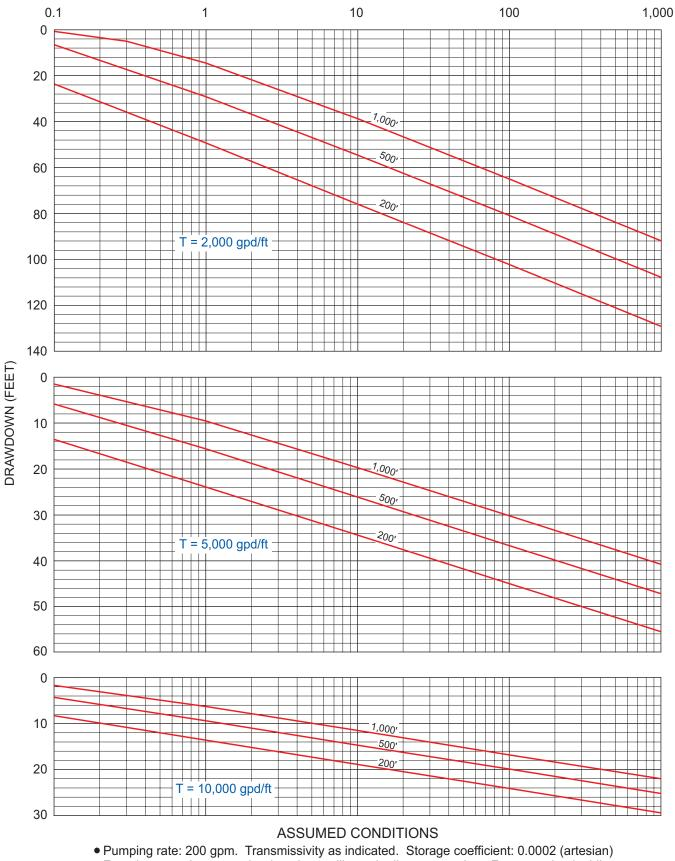
• For other pumping rates, the drawdown will vary in direct proportion. For example, doubling the pumping rate will double the drawdown at a given distance and time.
