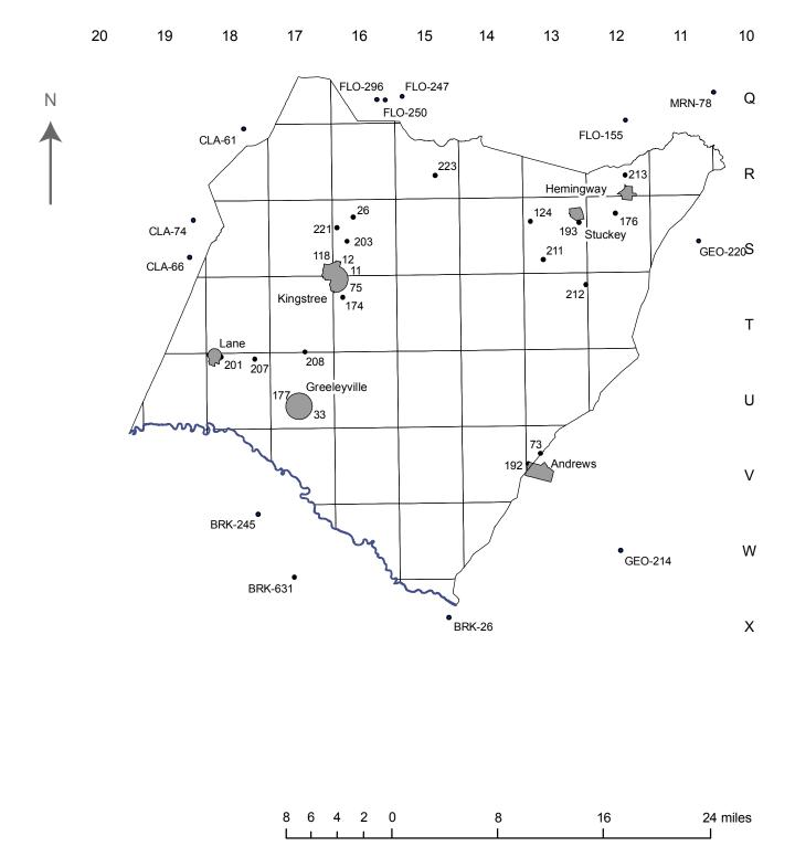
Figure 7. Wells for which pumping-test results are given in Table 3.
