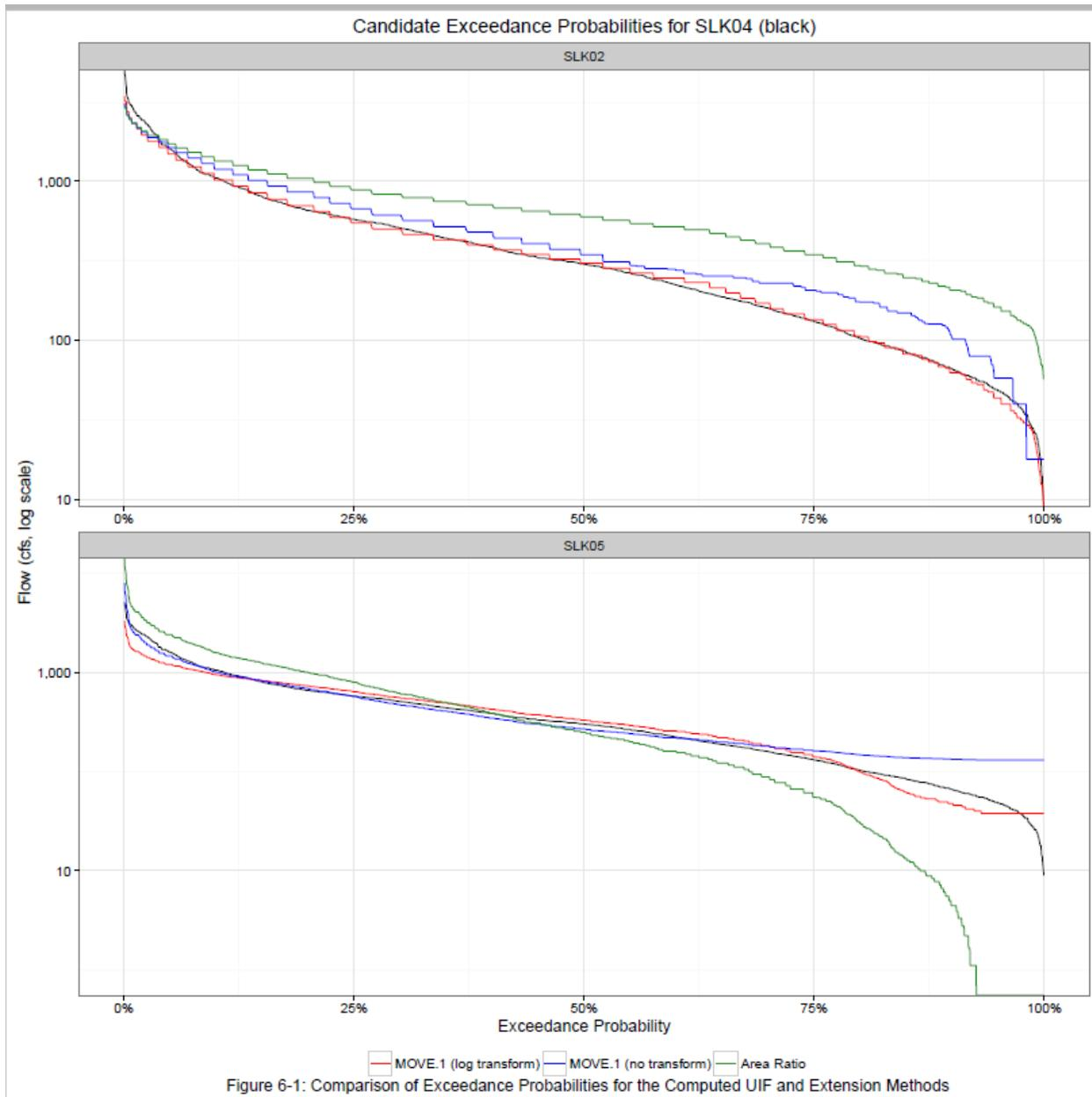
Figure 6-1: Comparison of Exceedance Probabilities for the Computed UIF and Extension Methods
