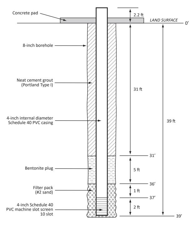
GEO-0386 well construction diagram.
