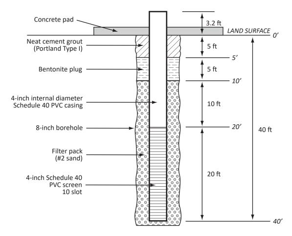
GEO-0391 well construction diagram.
