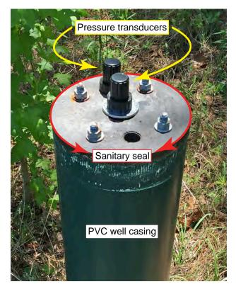
Figure 8. Pressure transducer installation at monitoring well HAM-0315 near Hampton, SC. Center probe measures water levels; rear probe measures barometric pressure.
