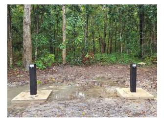
Figure 19. New monitoring wells at Myrtle Beach State Park in Horry County. HOR-1326 (left) is screened in the McQueen Branch aquifer (600 feet deep) and HOR-1327 (right) is screened in the Crouch Branch aquifer (440 feet deep). HOR-1327 is also part of the
