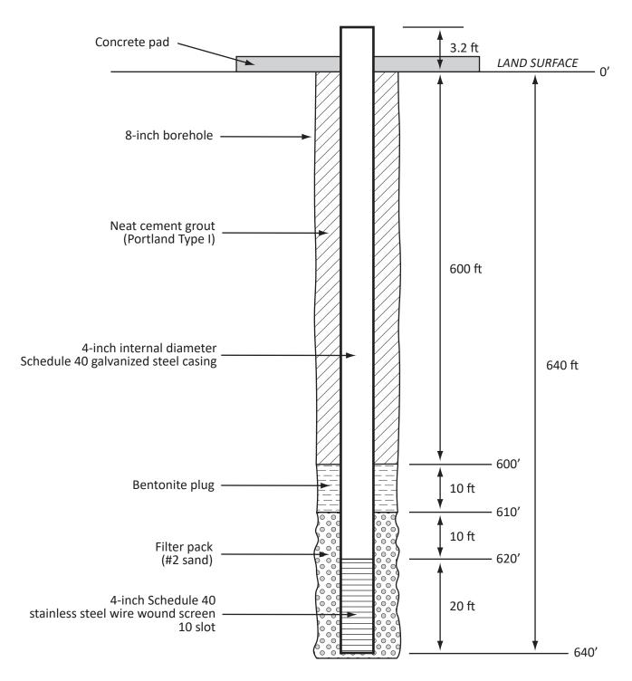
GEO-0390 well construction diagram.
