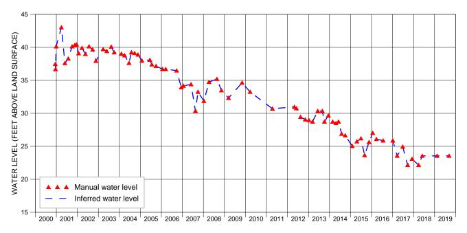
Figure 11. Manual water-level measurements in well MRN-0078 (Marion County). Because the water level in this well is above land surface, an ADR is not used, and measurements are made using a pressure test gage.
