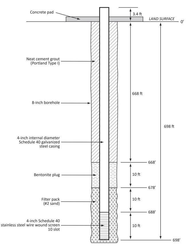
CAL-0215 well construction diagram.
