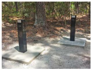
Figure 18. New monitoring wells at Hobcaw Barony in Georgetown County. GEO-0387 (left) is screened in the Gordon aquifer (95 feet deep) and GEO-0386 (right) is screened in the surficial aquifer (39 feet deep).
