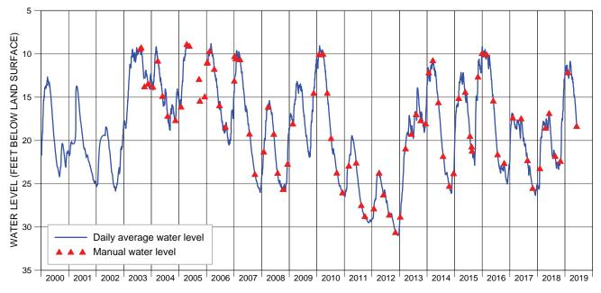
Figure 10. Daily average water levels in well SAL-0069 (Saluda County) calculated from hourly ADR data. Manual measurements made during site visits verify the accuracy of the ADR data.
