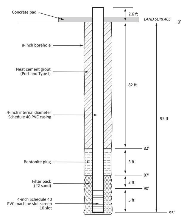
GEO-0387 well construction diagram.
