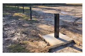
Figure 28. The new monitoring well CAL-0215, screened in the McQueen Branch aquifer, at the Creston cluster site. In the background are the four monitoring wells installed in 2014.
