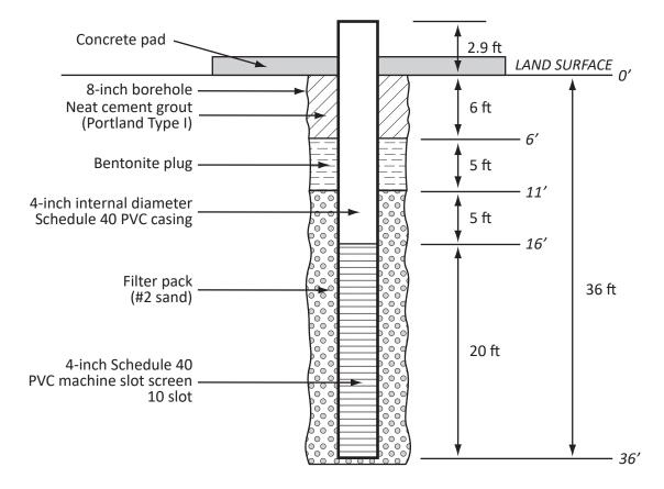
MRN-0178 well construction diagram.
