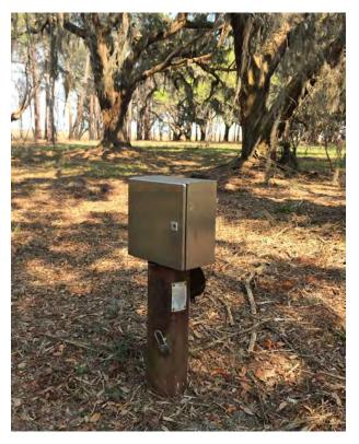
Figure 9. Saltwater Intrusion Monitoring Network well CHN-0803 at Santee Coastal Reserve, McClellanville, SC (Charleston County).
