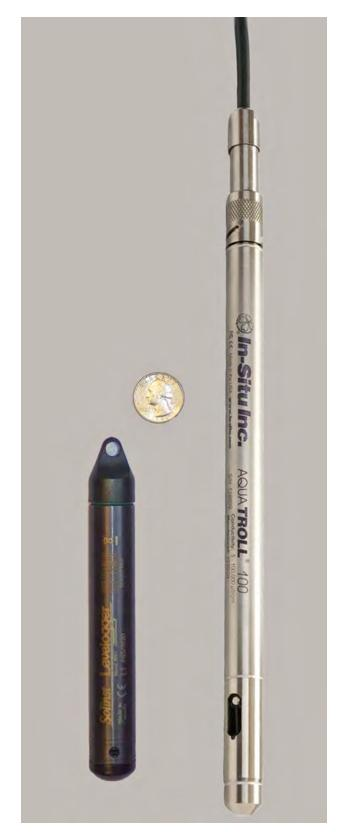
Figure 7. Two types of automated data recorders used in the SCDNR network: Solinst<sup>®</sup> Levelogger<sup>®</sup> (left) measures water-level; In-Situ<sup>®</sup> Aqua TROLL<sup>®</sup> (right) measures conductivity and temperature.
